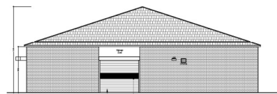
Side Elevation with Roller Shutter Closed SCALE 1/500 Roller shutter in closed position Preferred Section of Roller shutter to be confirmed
